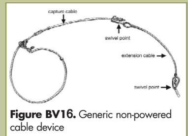
**Figure BV16.** Generic non-powered cable device
