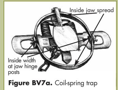
Figure BV7a. Coil-spring trap
