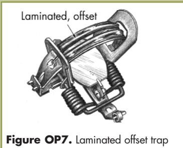
**Figure OP7.** Laminated offset trap
