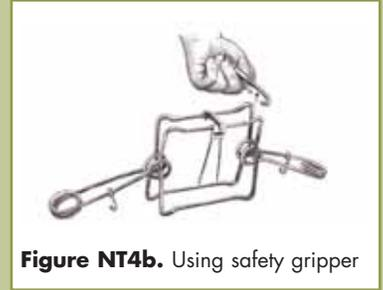
Figure NT4b. Using safety gripper
