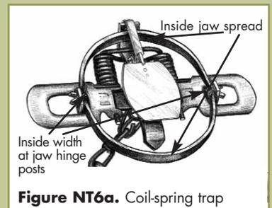
Figure NT6a. Coil-spring trap
