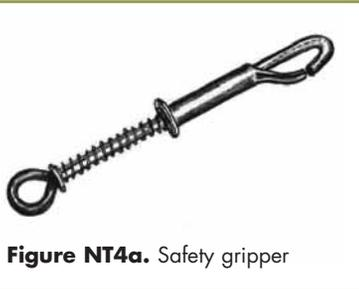
**Figure NT4a.** Safety gripper
