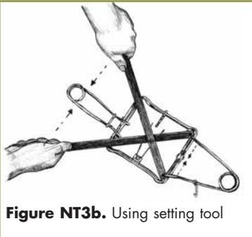
**Figure NT3b.** Using setting tool
