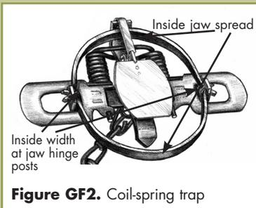
**Figure GF2.** Coil-spring trap
