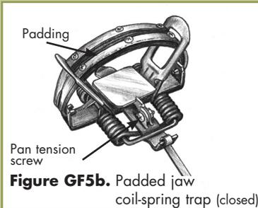
**Figure GF5b.** Padded jaw coil-spring trap (closed)
