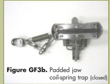
**Figure GF3b.** Padded jaw coil-spring trap (closed)
