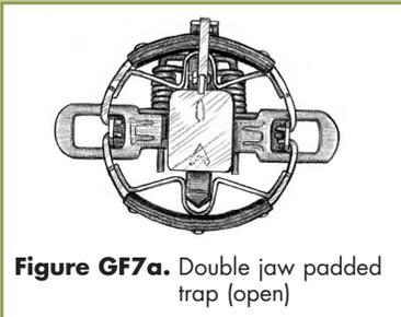
**Figure GF7a.** Double jaw padded trap (open)
