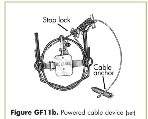
**Figure GF11b.** Powered cable device (set)
