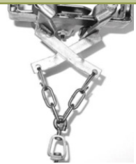
Figure WC19c. Compound levers
