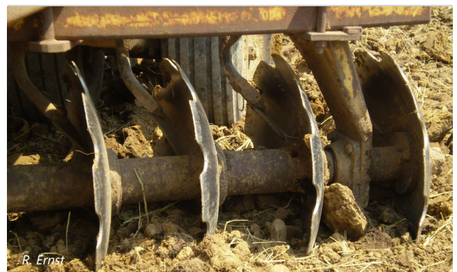
Figure 4-2: Example of disk plowing methods.
