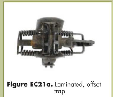
**Figure EC21a.** Laminated, offset trap
