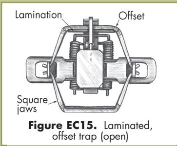
**Figure EC15.** Laminated, offset trap (open)
