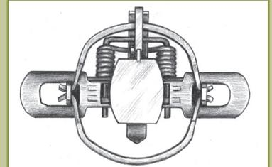
**Figure EC10a.** Unmodified jaw coil-spring trap (open)
