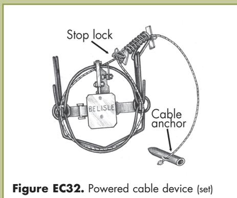
Figure EC32. Powered cable device (set)
