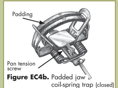
**Figure EC4b.** Padded jaw coil-spring trap (closed)
