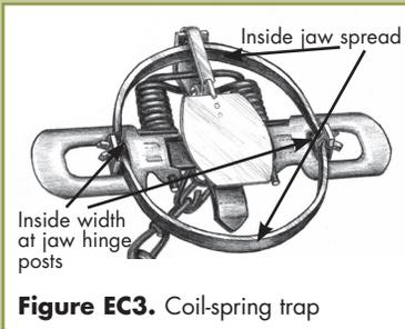
**Figure EC3.** Coil-spring trap
