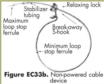
**Figure EC33b.** Non-powered cable device
