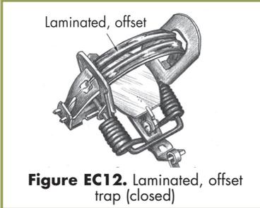
**Figure EC12.** Laminated, offset trap (closed)
