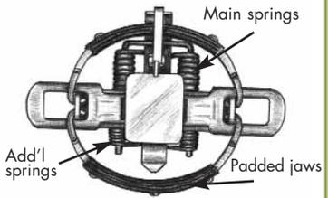
**Figure OP5a.** Padded jaw coil-spring trap (open)
