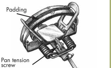
**Figure OP5b.** Padded jaw coil-spring trap (closed)
